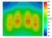
The figure on the left shows the temperature contour for the cooling channel of the cooling channel and its baseplate. It can be clearly seen that the coolant takes away the heat effectively keeping the temperature of the power module well within the limits.
