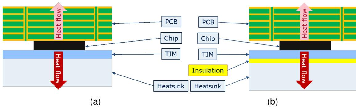
**Fig. 7:** Material stack-up without any electrical insulation and with electrical insulation.
