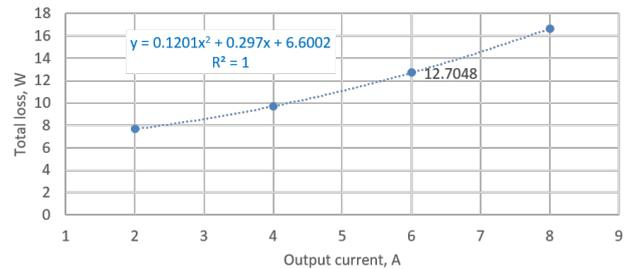
**Fig. 5:** Power loss estimated for the power transistors used in this application.
