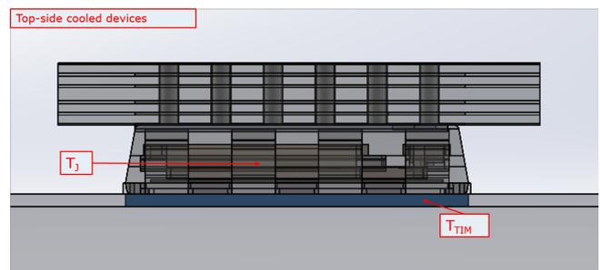
**Fig. 3:** Measuring point to evaluate the thermal resistance of a package.
