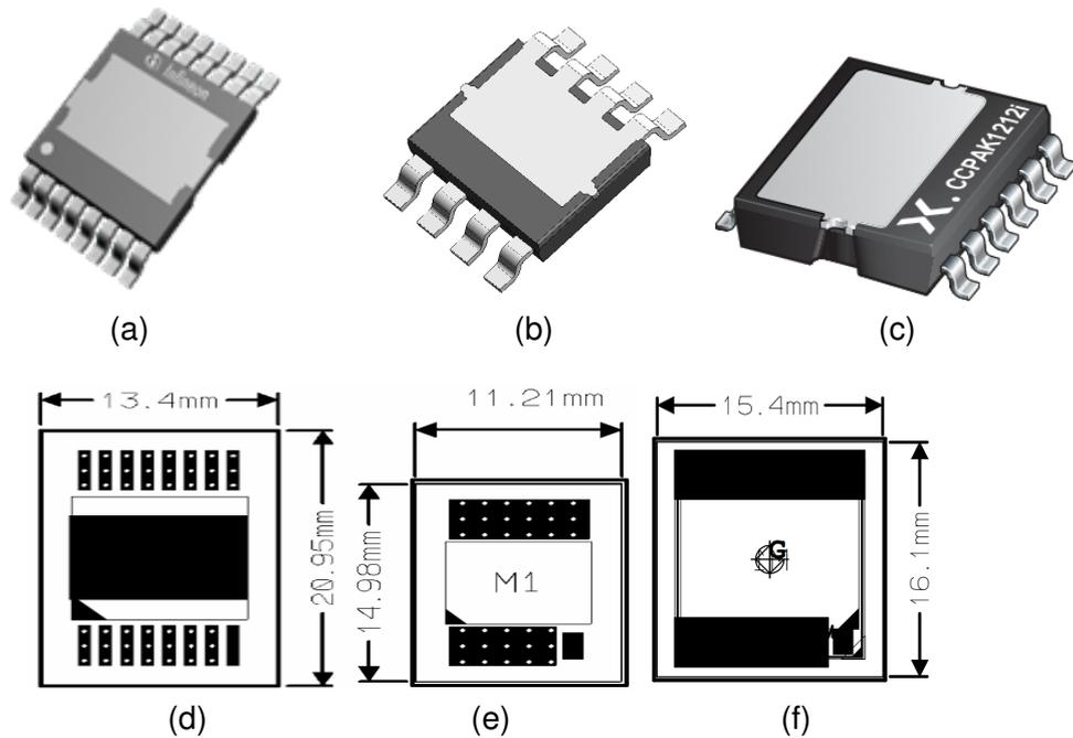
**Fig. 2:** Package under investigation: TOLT, PowerPAK® 8x8LR, and CCPAK1212i.
