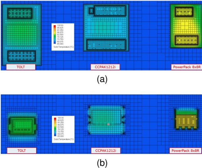
**Fig. 4:** Graphical visualization of the temperature of the three commercial packages under investigation (a) and of the respective TIM (b).
