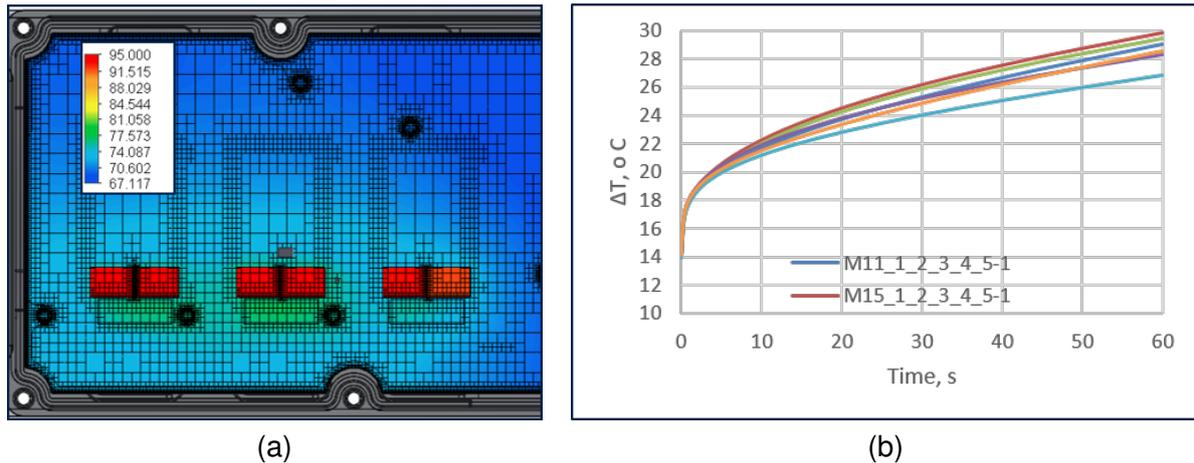
**Fig. 8:** CFD simulation for the transistors used (a) and the transient behavior for their junction temperatures (b).
