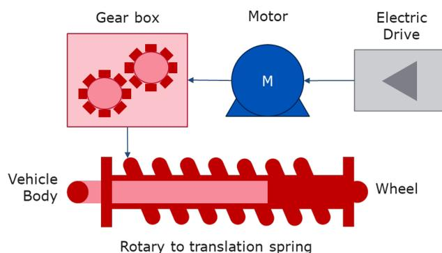
Fig. 1: Schematic structure of the leveling actuator.
